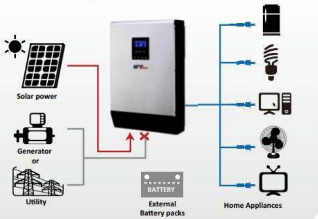
Solar Power available
